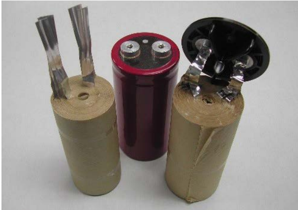
FIGURE 20: Aluminum electrolytic capacitors with windings composed of aluminum foils and cellulosic separators that exhibit thermal anisotropy.
